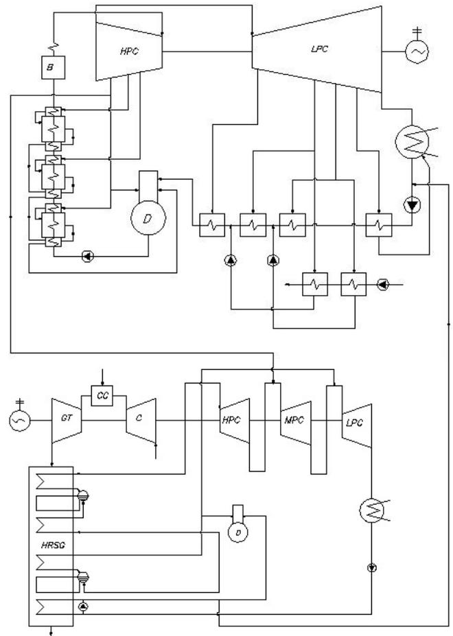
Figure 3: Thermal scheme of a hybrid energy complex based on a turbine with unclaimed industrial bleed-off
