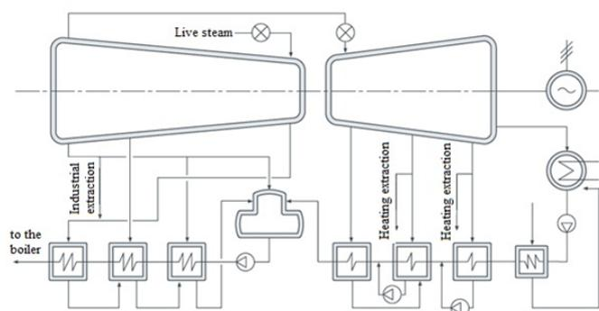
Figure 1: Thermal scheme of turbine PT-80-130
