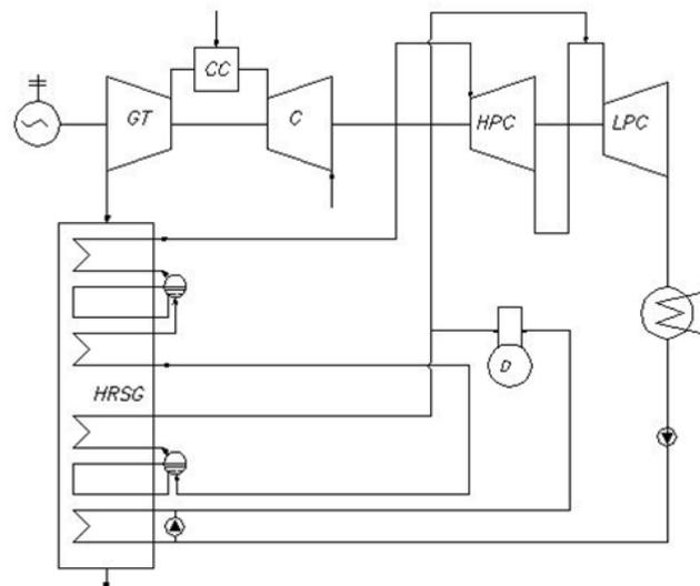
Figure 2: Thermal scheme of a single-shaft CCGT
