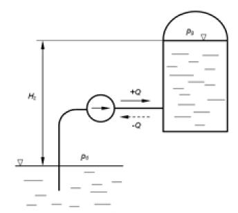
Figure 1: Positive (normal) and negative parameters of a working pump
