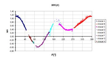
Figure 8:  $WH(\vartheta)$  for NHV50-250 pump (n<sub>q</sub>=15.6)
