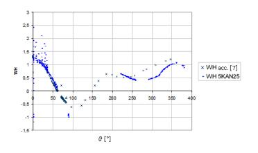
Figure 7:  $WM(\vartheta)$  for 5KAN25 pump (n<sub>q</sub>=11) against literature data (n<sub>q</sub>=35)
