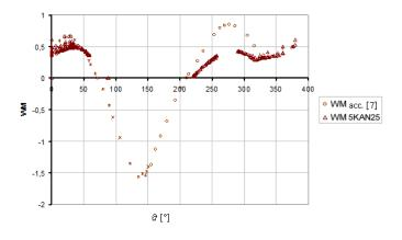
Figure 6:  $WH(\vartheta)$  for 5KAN25 pump (n<sub>q</sub>=11) against literature data (n<sub>q</sub>=35)
