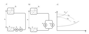
Figure 4: Two different pumps  $p_1$ ,  $p_2(p_1 \neq p_2$ connected in series (a) and in parallel (b), and pump and system characteristics (c);  $H_{uk,r}$ - system characteristics for pumps connected in parallel,  $H_{uk,s}$ - for pumps connected in series
