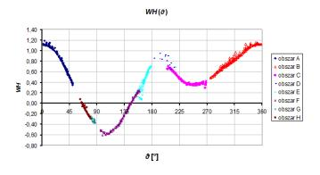
Figure 9:  $WM(\vartheta)$  for NHV50-250 pump (n<sub>a</sub>=11)
