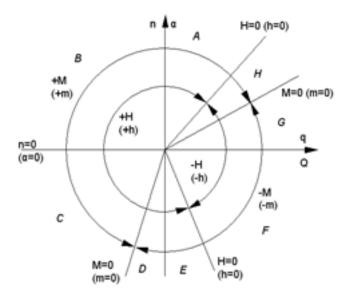
Figure 3: Possible pump functioning areas A÷H
