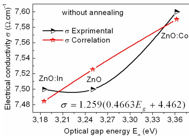
Figure 4: The correlation between electrical conductivity  $\sigma$  and optical band gap energy  $E_g$  for ZnO, ZnO:In and ZnO:Co thin films without annealing
