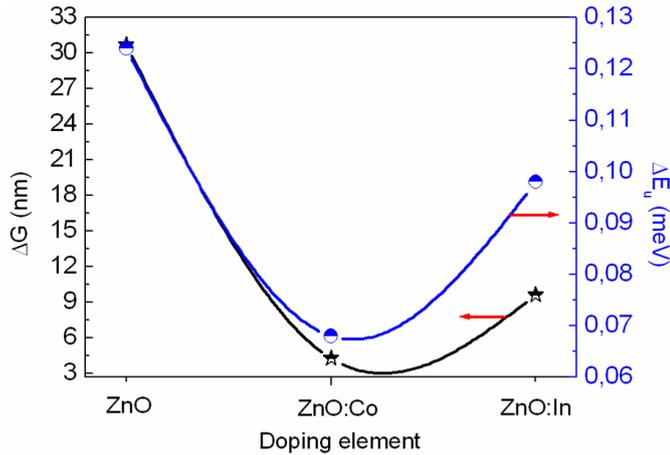
Figure 1: The variation of the difference in crystallite size ( $\Delta G$ ) with the difference in Urbach energy ( $\Delta E_u$ ) of ZnO, ZnO:In and ZnO:Co thin films
