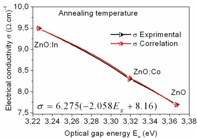
Figure 5: The correlation between electrical conductivity  $\sigma$  and optical band gap energy  $E_g$  for ZnO, ZnO:In and ZnO:Co thin films for annealing temperature at 500°C
