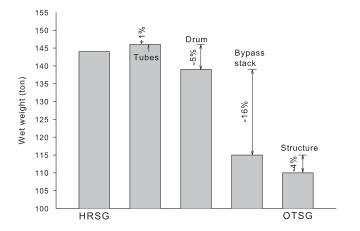
Figure 3: Breakdown of wet weight difference between a drumtype and a once-through HRSG for offshore applications
