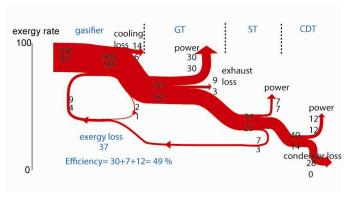
Figure 9: Energy/Exergy flow of the IGCC model
