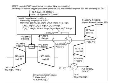
Figure 8: Performance and process flow diagram of the A-IGCC model
