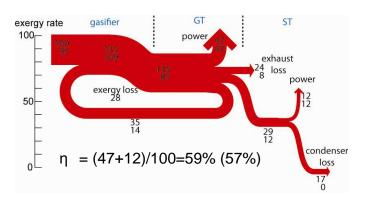
Figure 4: Theoretical energy/exergy flow of the Advanced IGCC system with exergy recuperation [6]. The net efficiency in brackets takes oxygen generation power into consideration.
