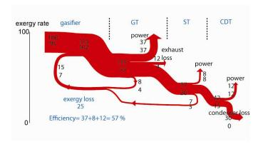
Figure 10: Energy/Exergy flow of the A-IGCC model
