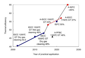
Figure 1: Performance projection of future coal based power plants [6]
