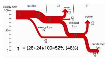
Figure 3: Theoretical energy/exergy flow of a conventional cascading IGCC system [6]. The net efficiency in brackets takes oxygen generation power into consideration.
