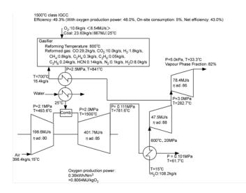
Figure 7: Performance and process flow diagram of IGCC model
