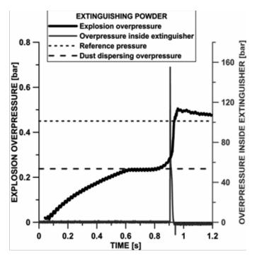
Figure 11: Courses of the overpressure inside the 1.3 m<sup>3</sup> test chamber during explosion of corn starch dust (C = 0.2 kg/m<sup>3</sup>) and inside the extinguisher. Activation from photodiode signal at the level of 0.6 V. Explosion overpressure  $\Delta P = 0.055$  bar
