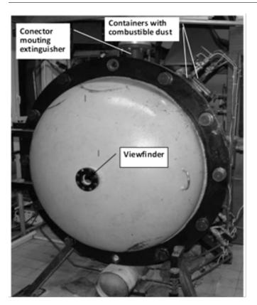
Figure 2: Explosion chamber with 1.3 m<sup>3</sup> volume
