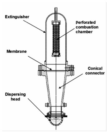
Figure 7: Schematic diagram of the extinguisher
