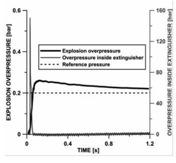
Figure 14: Courses of the overpressure inside the 1.3 m<sup>3</sup> test chamber during explosion of a methane-air mixture (7.5% CH<sub>4</sub>). Activation from photodiode signal at the level of 0.3 V. Explosion overpressure  $\Delta P = 0.06$  bar
