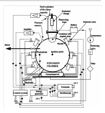
Figure 3: Schematic diagram of the research stand with 1.3  $\rm m^3$  explosion chamber – for dust explosion investigations
