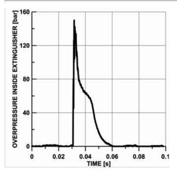
Figure 19: Example course in fire extinguisher pressure recorded during the test explosion suppression
