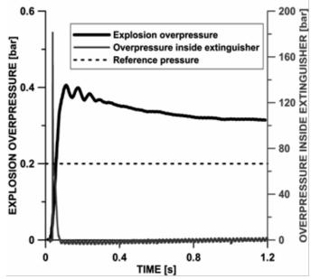
Figure 16: Courses of the overpressure inside the 1.3 m<sup>3</sup> test chamber during explosion of a methane-air mixture (7.5% CH<sub>4</sub>). Activation from photodiode signal at the level of 1.0 V. Explosion overpressure  $\Delta P = 0.21$  bar
