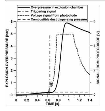
Figure 9: Courses of the overpressure inside test chamber and photodiode voltage signal obtained during explosion of the corn starch dust (C =  $0.2 \text{ kg/m}^3$ ), without suppression. Explosion overpressure  $\Delta P = 5.7$  bar
