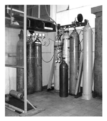
Figure 4: General view of the stand for precise preparation of the tested gaseous mixtures
