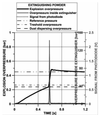
Figure 10: Courses of the overpressure inside the 1.3 m<sup>3</sup> test chamber during explosion of corn starch dust  $(C = 0.2 \text{ kg/m}^3)$  and inside the extinguisher. Activation from photodiode signal at the level of 0.3 V. Explosion overpressure  $\Delta P = 0.035$  bar
