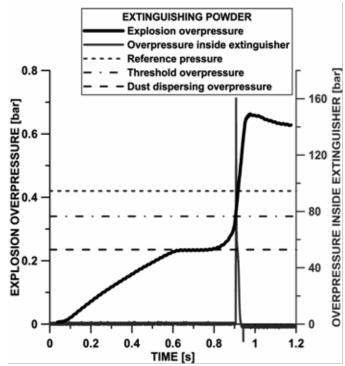
Figure 12: Courses of the overpressure inside the 1.3 m<sup>3</sup> test chamber during explosion of corn starch dust  $(C = 0.2 \text{ kg/m}^3)$  and inside the extinguisher. Activation from photodiode signal at the level of 1.0 V. Explosion overpressure  $\Delta P = 0.24$  bar
