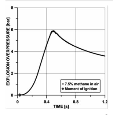
Figure 13: Courses of the overpressure inside the 1.3 m<sup>3</sup> test chamber during explosion of a methane-air mixture  $(7.5\% \text{ CH}_4)$
