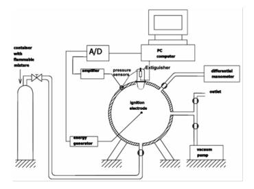
Figure 6: Schematic diagram of the research stand with 1.3  $\rm m^3$  explosion chamber – for investigation of gaseous explosion suppression
