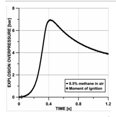
Figure 17: Courses of the overpressure inside the 1.3 m<sup>3</sup> test chamber during explosion of a methane-air mixture  $(8.5\% \text{ CH}_4)$
