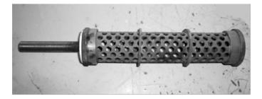
Figure 8: View of the perforated steel combustion chamber
