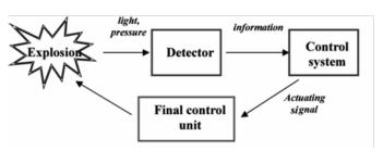
Figure 1: Principle of operation of the suppression system
