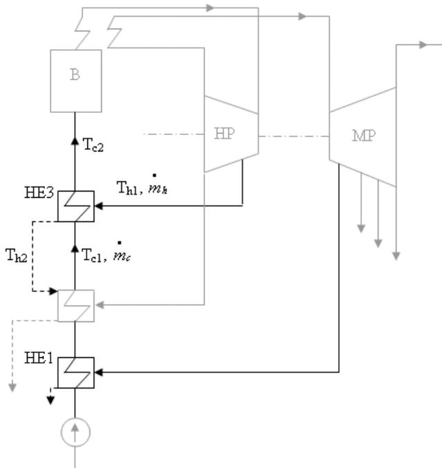
Figure 1: Location of the analyzed regenerative heat exchangers in a 200 MW power plant
