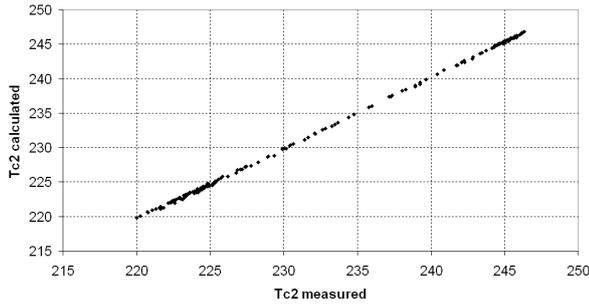
Figure 2: A comparison between water temperature at the outlet of the heat exchanger, measured and calculated (for the HE3 heat exchanger)
