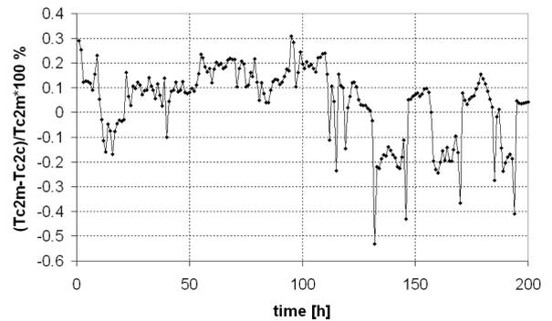
Figure 12: Relative difference between water temperature at the outlet of the heat exchanger, measured (m) and calculated (c) in % (for the HE1 heat exchanger)
