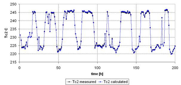
Figure 4: Change of water temperature at the outlet of the heat exchanger, measured and calculated (for the HE3 heat exchanger)
