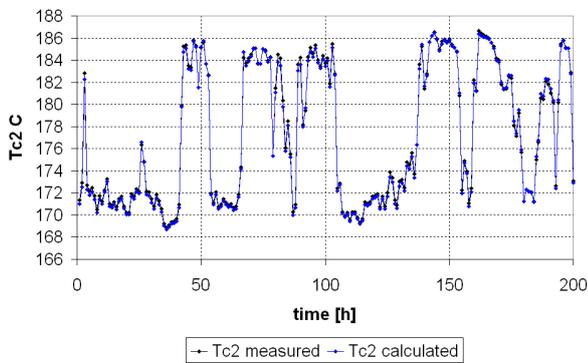
Figure 14: Change of water temperature at the outlet of the heat exchanger, measured and calculated (for the HE1 heat exchanger) for data at the end of the year
