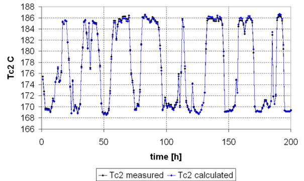
Figure 11: Change of water temperature at the outlet of the heat exchanger, measured and calculated (for the HE1 heat exchanger)
