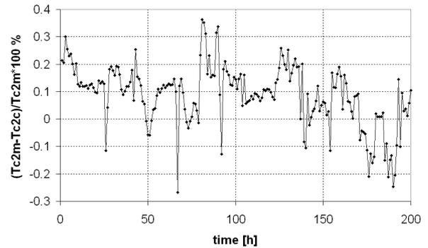
Figure 15: Relative difference between water temperature at the outlet of the heat exchanger, measured (m) and calculated (c) in % (for the HE1 heat exchanger) for data at the end of the year
