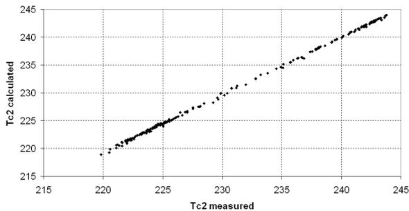
Figure 6: Comparison between water temperature at the outlet of the heat exchanger measured and calculated (for the HE3 heat exchanger) for data at the end of the year
