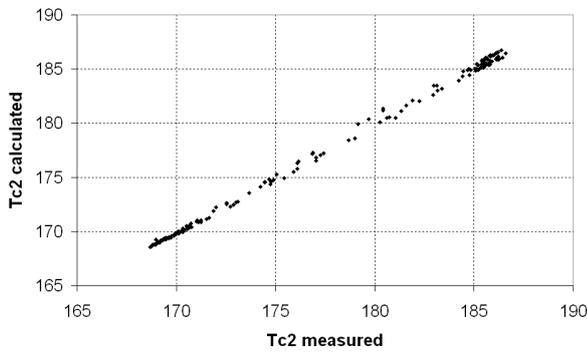
Figure 10: A comparison between water temperature at the outlet of the heat exchanger, measured and calculated (for the HE1 heat exchanger)
