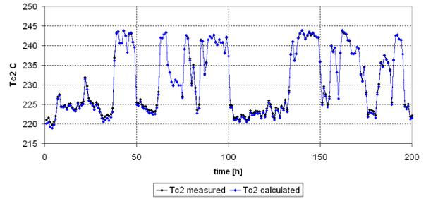
Figure 7: Change of water temperature at the outlet of the exchanger measured and calculated (for the HE3 heat exchanger) for data at the end of the year
