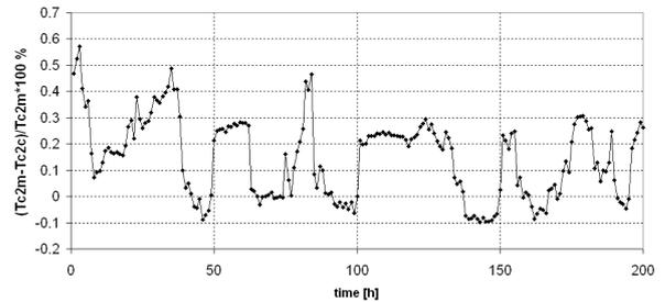
Figure 8: Relative difference between water temperature at the outlet of the heat exchanger, measured (m) and calculated (c) in % (for the HE3 heat exchanger) for data at the end of the year
