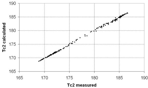
Figure 13: A comparison between water temperature at the outlet of the heat exchanger measured and calculated (for the HE1 heat exchanger) for data at the end of the year
