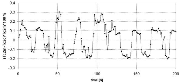
Figure 5: Relative difference between water temperature at the outlet of the heat exchanger, measured (m) and calculated (c) in % (for the HE3 heat exchanger)
