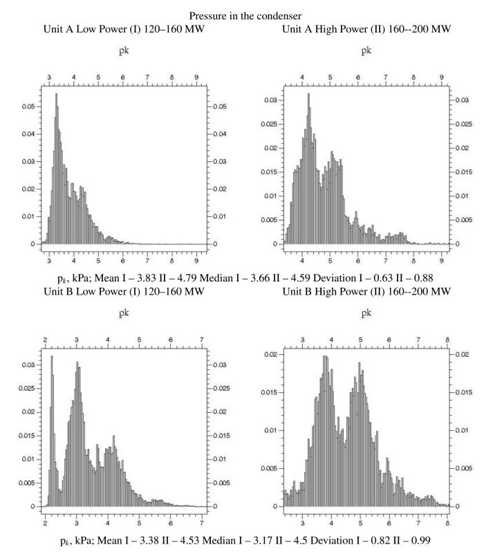
Figure 4: Histograms of pressure in the condenser
