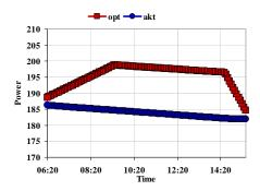
Figure 10: The track of power changes in a commercial CHP plant for normally applied (act) and optimal (opt) load distributions
