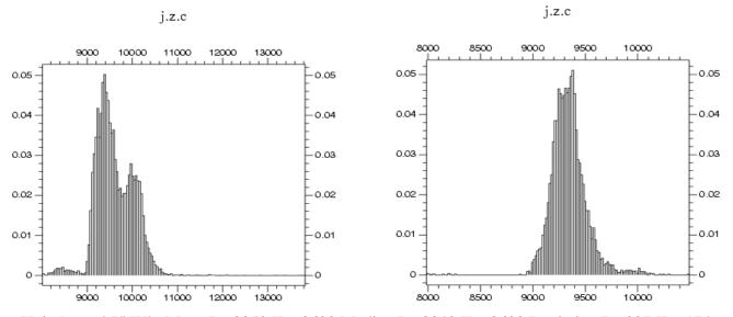
Unit A, q<sub>b</sub>, kJ/kWh; Mean I – 8850 II – 8630 Median I – 8840 II – 8638 Deviation I – 397 II – 174 Unit B Low Power (I) 120--160 MW Unit B High Power (II) 160--200 MW
