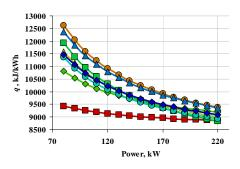
Figure 8: Characteristics of unit heat consumption for "identical" units installed in the same power plant
