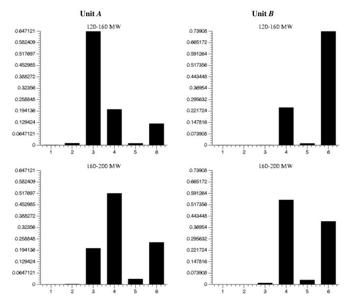
Figure 5: Results of data analysis by the PCA method; 1 -live steam pressure, 2 -live steam temperature, 3 -pressure drop in the superheater, 4 -temperature of secondary superheated steam, 5 -pressure in the condenser, 6 -temperature of supply water, 7 -amount of oxygen in flue gases, 8 -flue gases temperature
