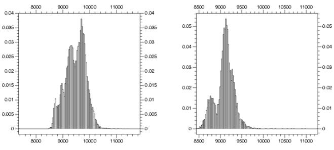
Unit B, q<sub>b</sub>, kJ/kWh; Mean I – 8756 II – 8107 Median I – 8787 II – 8425 Deviation I – 353 II – 214
