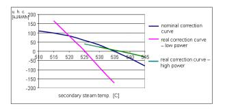
Figure 6: Correction curve  $\triangle q_b$  for secondary steam temperature and corresponding curves resulting from statistical analysis of a real unit
