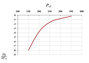
Figure 7: Derivative of unit chemical energy consumption of a fuel in the function of the unit power
