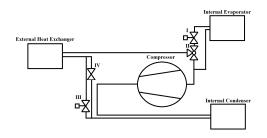
Figure 1: Nissan Leaf heating-cooling system diagram ( I III expansion valve, II three-way valve , IV bypass )
