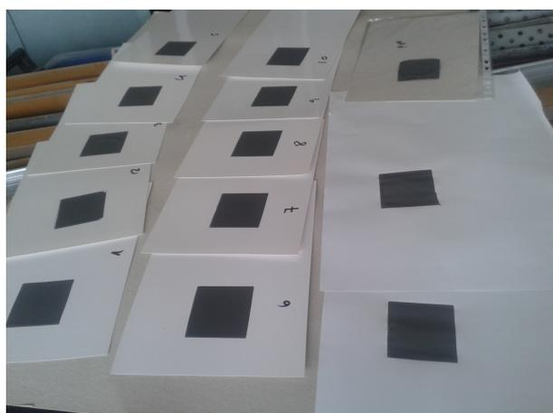
Figure 9: Molten Carbonate Fuel Cell cathode layers screen-printed on various substrates
