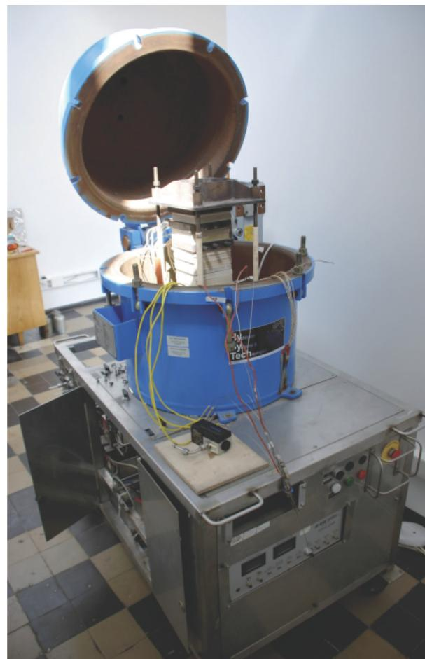
Figure 11: Stand for testing high-temperature fuel cells at Warsaw University of Technology
