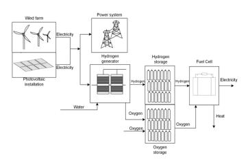
Figure 1: Schematic diagram of a Power to Gas to Power installation
