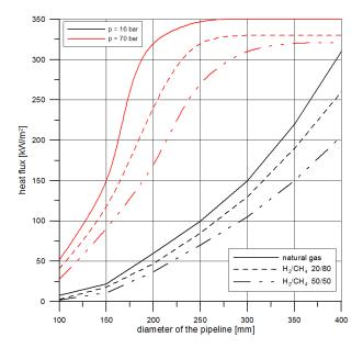
Figure 13: Heat flux depending on distance from the fire site (puncture damage to the pipeline)
