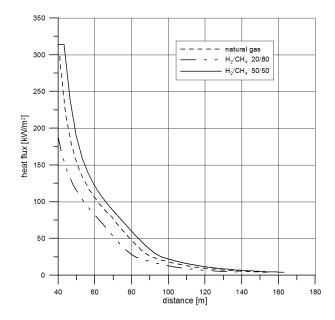
Figure 10: Heat flux depending on the distance from the fire (full-bore rupture)
