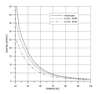
Figure 11: Heat flux depending on the distance from the fire (puncture damage)
