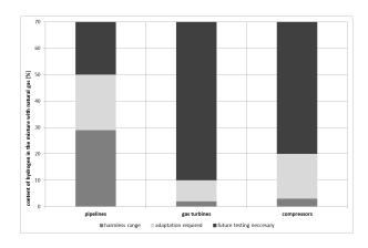
Figure 1: Impact of the content of hydrogen in the mixture with natural gas on the transmission system elements [9]
