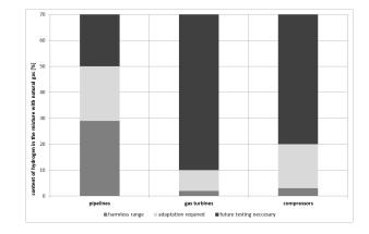
Figure 2: Impact of the content of hydrogen in the mixture with natural gas on selected elements of the distribution system [9]
