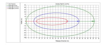
Figure 6: Hazard zones related to methane jet fire
