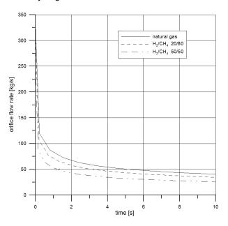
Figure 8: Mass flow of released substance depending on time-full-bore rupture
