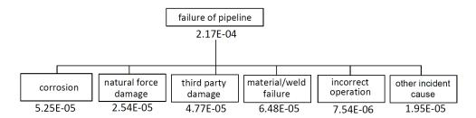
Figure 4: Rate of the occurrence of damage to pipelines
