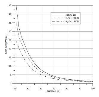
Figure 12: Heat flux depending on distance from the fire site (puncture damage to the pipeline)
