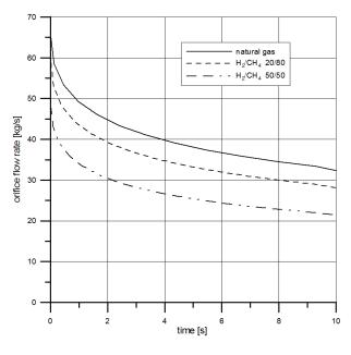
Figure 9: Mass flow of released substance depending on time-puncture damage
