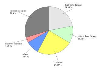
Figure 3: Causes of pipeline damage
