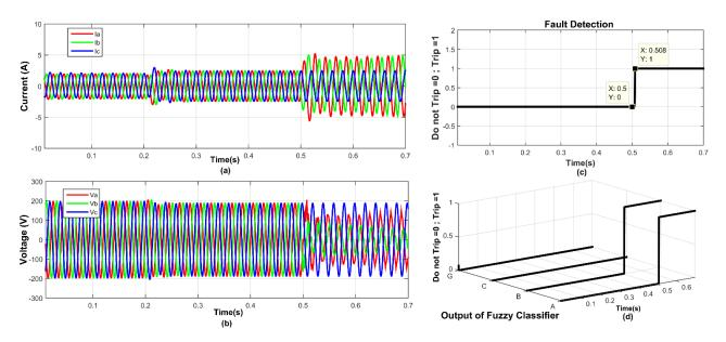
Figure 7: Performance during LL fault (a) Current (b) Voltage (c) Fault detection (d) Fault classification
