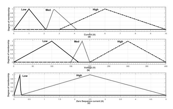
Figure 4: Degree of fuzzy membership function for input variable (a) current for phase fault detection (b) voltage for phase fault detection (c) zero sequence current for ground fault detection
