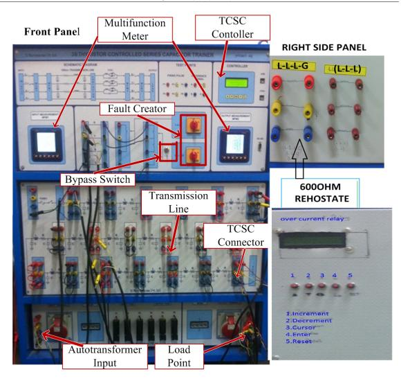
Figure 1: Prototype Model of TCSC Connected 180km long Transmission Line
