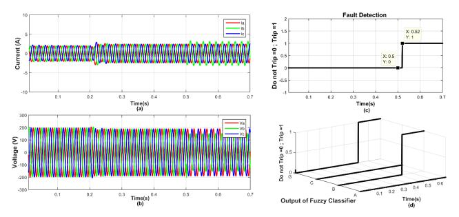
Figure 6: Performance during BG internal fault at remote end (a) Current Signals (b) Voltage Signals (c) Fault detection (d) Fault classification
