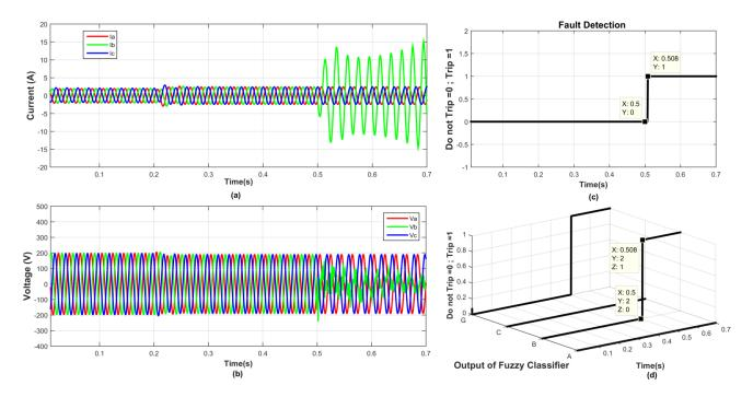
Figure 5: Performance during BG internal fault at near end (a) Current Signals (b) Voltage Signals (c) Fault detection (d) Fault classification
