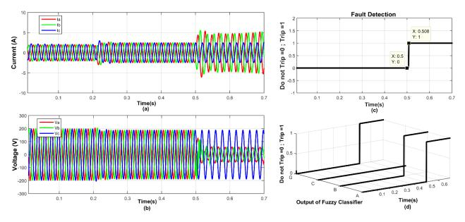
Figure 8: Performance during LLG fault (a) Current (b) Voltage (c) Fault detection (d) Fault classification
