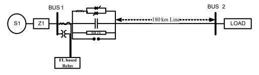
Figure 2: Single line diagram of TCSC compensated transmission network
