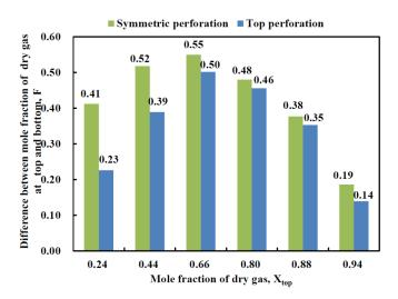
Figure 12: Histogram of the value of F with mole fraction of dry gas at the top formation under symmetric perforation and top perforation of the reservoir
