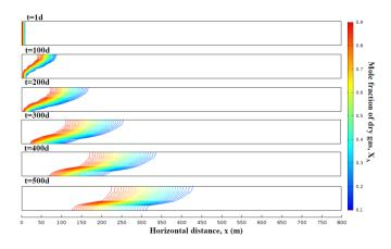
Figure 3: Isoline changes of the mole fraction distribution of dry gas in the rectangular region with time
