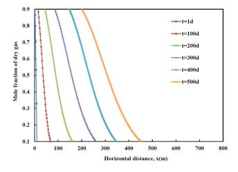
Figure 4: Variation curves of the mole fraction of dry gas at the middle position with the horizontal distance at different times
