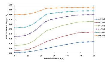
Figure 7: Relation curves of the mole fraction of dry gas and the vertical distance at different times
