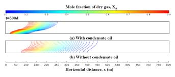
Figure 9: Isoline of the mole fraction distribution of dry gas in the rectangular region with and without condensate oil
