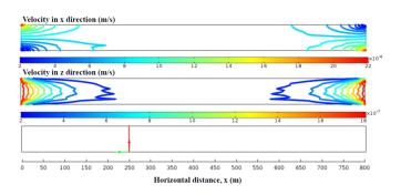
Figure 6: Isoline of velocity distribution on the x and z-directions in the rectangular region and the cutting line at x = 250 m
