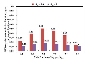
Figure 10: Histogram of the value of F with the mole fraction of dry gas at the top formation with and without condensate oil
