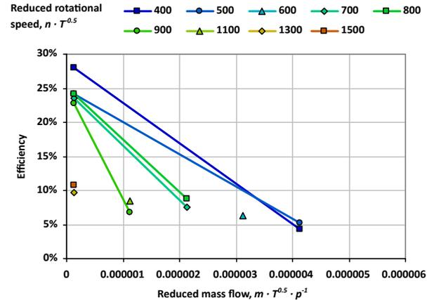
Figure 15: Efficiency curves for expander operated on air as functions of reduced mass flow,  $\frac{\dot{m} \cdot \sqrt{T}}{p}$  for various reduced rotational speeds,  $\frac{n}{\sqrt{T}}$
