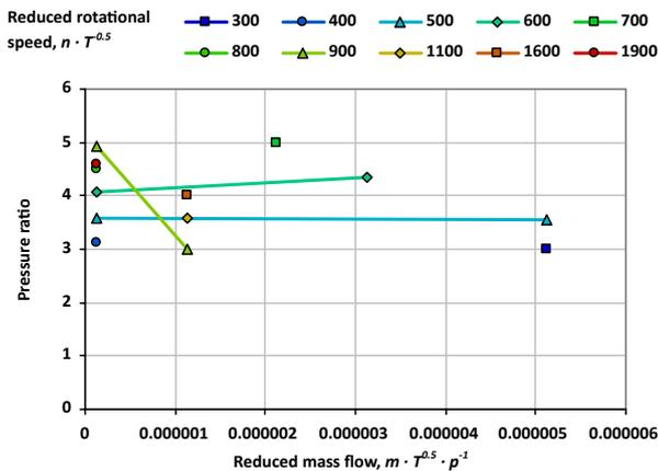
Figure 14: The expander operated on carbon dioxide pressure ratio as a function of reduced mass flow,  $\frac{\dot{m} \cdot \sqrt{T}}{p}$  for various reduced rotational speeds,  $\frac{n}{\sqrt{T}}$
