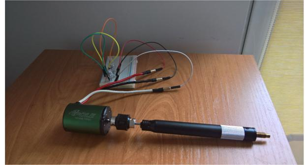
Figure 11: The expander-generator set used for the experiments
