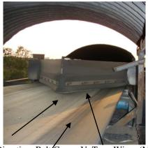
Direction Belt Conv V Type Wiper (M.S. Plate) Figure 3: Wiper installed on BC
