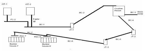
Figure 5: Single stream conveyor system at new NP TPS
