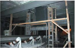
Figure 10. Support for Gravity take-up Arrangement
