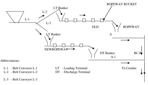
A - Belt Conveyor A, A-2 - Belt Conveyor A-1, BC-B- Belt Conveyor –B
