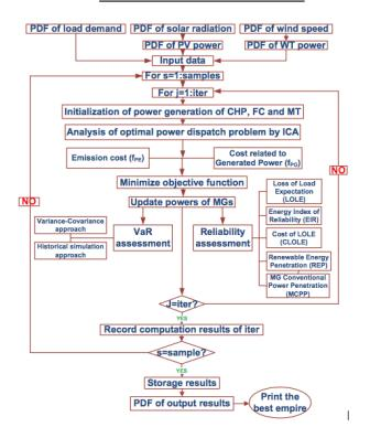
Figure 2: Flowchart of the ICA on probabilistic power dispatch considering reliability and VaR assessments
