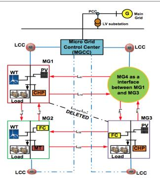
Figure 1: Structure of future smart distribution grid with NMGs
