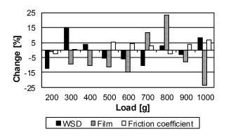
Figure 5: Change in lubricating properties for mix2 compared with ESSO-MARCOL
