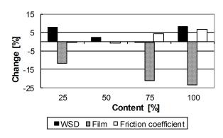
Figure 7: Change in lubricating properties depending on mix2 content in ESSOMARCOL oil
