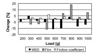
Figure 4: Change in lubricating properties for mix1 compared with ESSO-MARCOL
