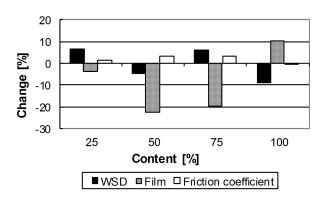
Figure 6: Change in lubricating properties depending on mix1 content in  $\ensuremath{\mathsf{ESSOMARCOL}}$  oil
