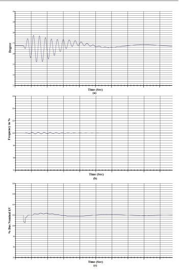
Figure 6: (a) Relative power Angle in Deg Vs Time in Sec. for generators G1 & G2, (b) % of Gen. Bus Frequency Vs Time in Sec for generators G1 & G2, (c) % of Gen Bus Voltage Vs Time in Sec for generators G1 & G2
