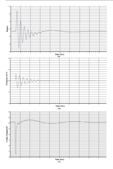
Figure 5: (a) Relative power Angle in Deg Vs Time in Sec. for generators G1 & G2, (b) % of Gen. Bus Frequency Vs Time in Sec for generators G1 & G2, (c) % of Gen Bus Voltage Vs Time in Sec for generators G1 & G2
