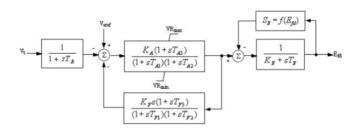
Figure 2: IEEE Type-AC5A excitation model
