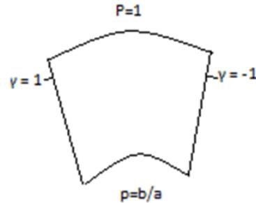
Figure 5: Non-Dimensional Arc element
