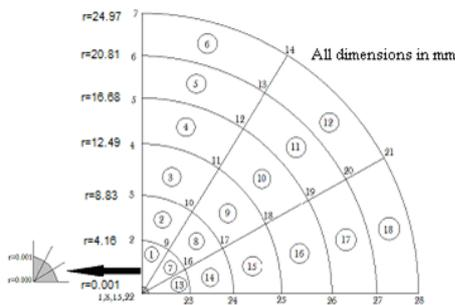
Figure 2: Slice of core conductor delimited by two 90° inclined planes divided into arc formed components
