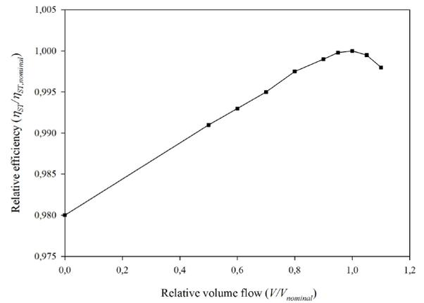
Figure 3: ST efficiency correction characteristic
