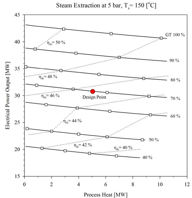
Figure 6: Calculated operational chart for extraction of steam at  $T_s = 150^\circ\text{C}$
