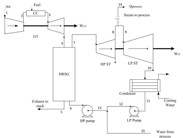
Figure 1: Layout of extraction steam turbine cycle
