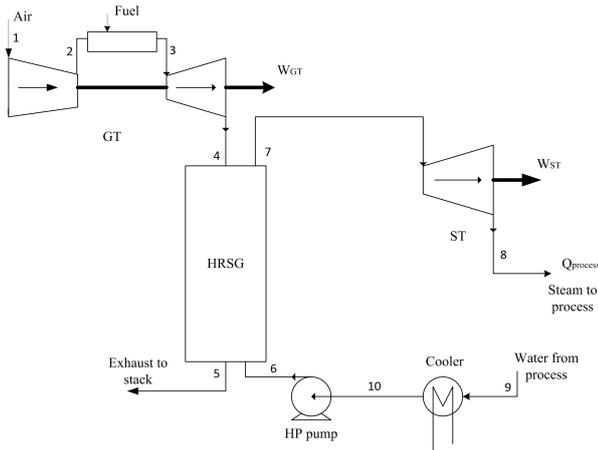
Figure 2: Layout of backpressure steam turbine cycle
