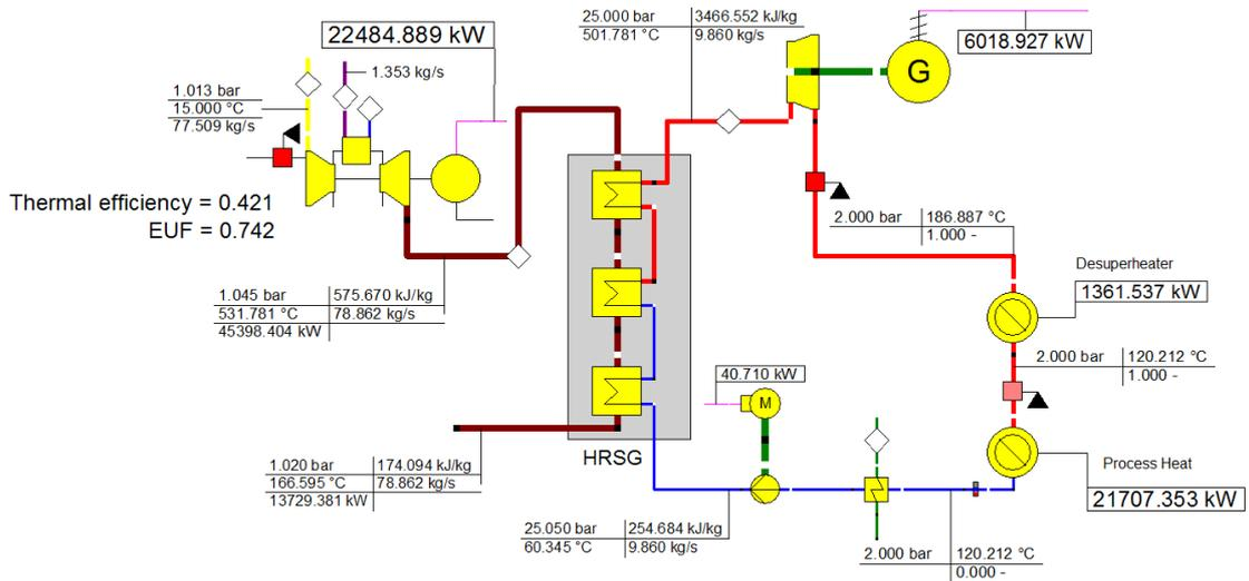
Figure 5: Layout of backpressure steam turbine cycle
