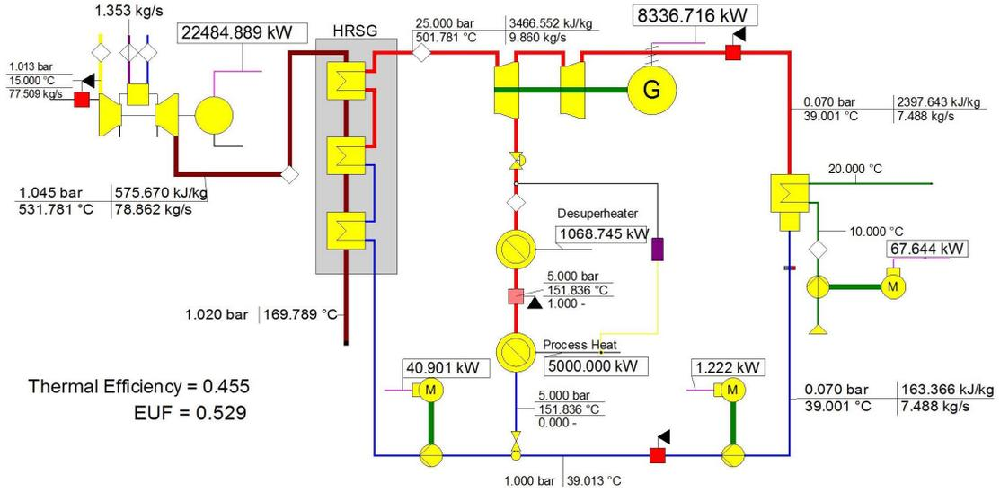
Figure 4: Layout of extraction steam turbine cycle
