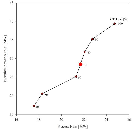
Figure 7: Operational line for backpressure steam turbine at 2 bar
