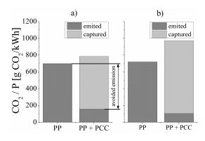
Figure 8: Comparison of amount of  $CO_2$  produced in the installation with and without PCC, IMC results (a) and data taken from work [35] (b), both figures share the same scale
