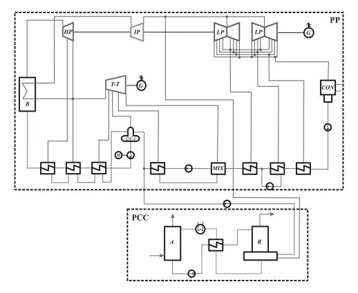
Figure 1: Object of the research – power plant coupled with a CO2 separation unit
