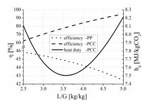
Figure 2: CO<sub>2</sub> capture and PP efficiencies and heat duty vs L/G.
