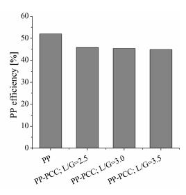
Figure 5: PP efficiency with and without PCC
