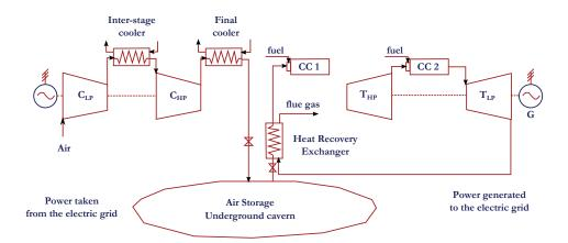
Figure 6: The operating principle and basic elements of the CAES power plant:  $C_{LP}$ ,  $C_{HP}$ —low pressure and high pressure compressors, respectively;  $T_{HP}$ ,  $T_{LP}$ —high pressure and low pressure part of the turbine, respectively; CC 1, CC 2—combustion chamber
