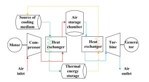
Figure 9: Schematic diagram of an Advanced Adiabatic–CAES system [45]
