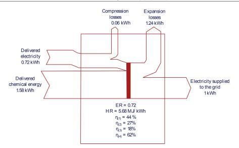
Figure 17: Sankey diagram showing the main flows of energy during charging and discharging processes. It also shows the efficiencies of the whole cycle in accordance with the definitions
