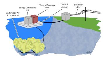
Figure 4: An Under Water CAES with on-shore equipment [35]
