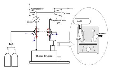
Figure 3: A hybrid pneumatic combustion engine [34]
