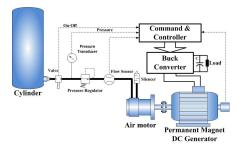
Figure 2: Pneumatically-driven electric generator of a stand-alone small scale CAES [31]
