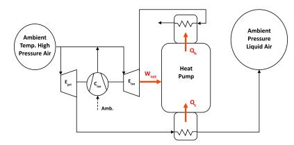
Figure 5: Schematic for the ideal (reversible) hybrid liquid air—CAES [40]
