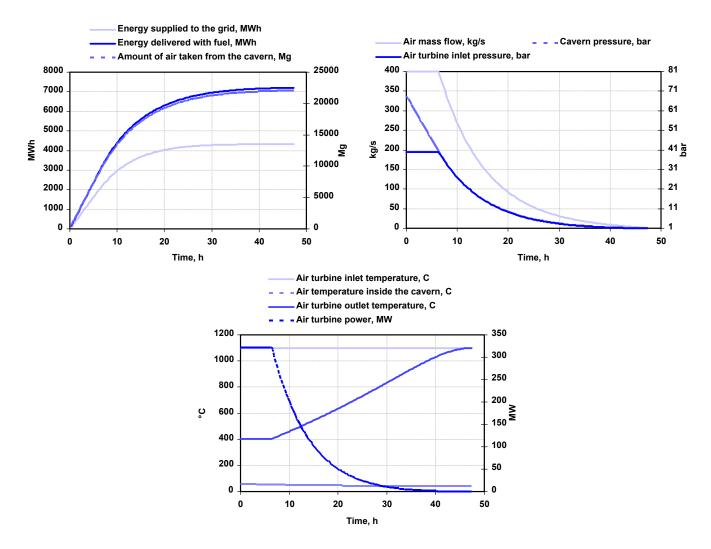
Figure 19: The main parameters of the discharging process from 70 to 1 bar with heating air to 1,100°C at turbine inlet
