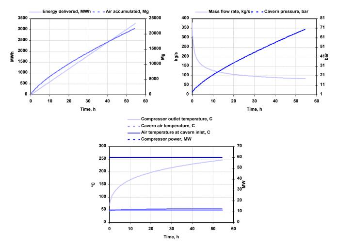
Figure 18: The main parameters of the charging process from 1 to 70 bar
