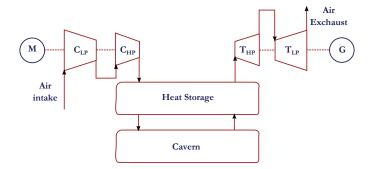
Figure 8: Working principles of an adiabatic CAES plant
