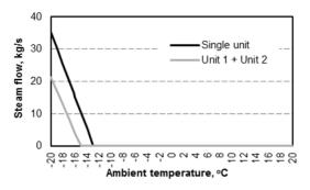
Figure 7: Relation between volume of steam used to feed into XC5 heater for steam extraction from one and two power units (for steam bleed from two units the feed into XC5 heater
