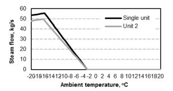
Figure 10: Relation between steam flow into XC3 heater and ambient temperature for heater feeding from one and two power units
