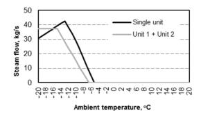
Figure 6: Relation between volume of steam used to feed into XC4 heater for steam extraction from one and two power units (for steam extraction from two power units the feed into XC4 heater is the sum of steam flow into XC4.1 and XC4.2 heaters)
