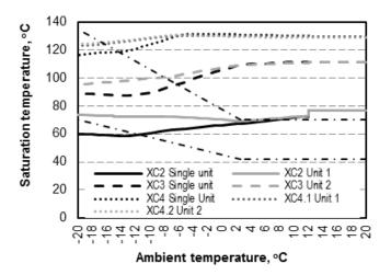
Figure 3: Relation between saturation temperature before XC2, XC3, XC4 (XC4.1, XC4.2) heaters and ambient temperature for steam bleed from one and two units used to feed heaters
