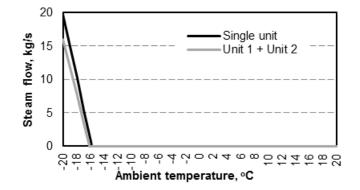
Figure 11: Relation between extraction steam flow into XC4 heater and ambient temperature for heater feeding from one and two power units (for steam extraction from two units the volume extracted into XC4 is made up by the total of flows into XC4.1 and XC4.2)
