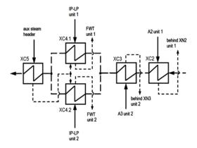
Figure 2: Configuration of heaters with steam bleed from two power units
