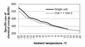
Figure 12: Relation between specific use of chemical energy of fuel and ambient temperature for steam feeding from one and two power units into the heaters (power unit operating at the output of 180 MW)
