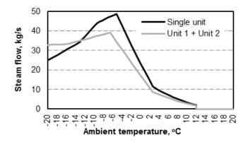
Figure 5: Relation between steam extraction into XC3 heater for feeding this heater from one and two power units
