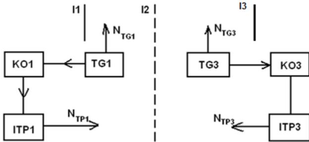
Figure 1: Configuration composed of several ( $i=1-3...$ ) double-shaft systems: TG (the gas turbine set) + KO (waste heat boiler) + ITP (steam turbine installation)
