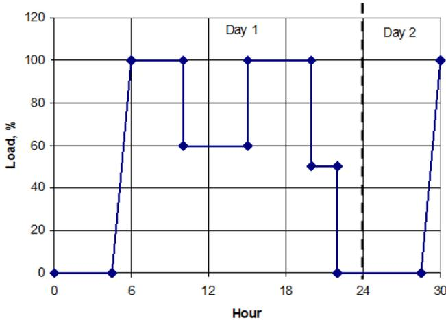
Figure 6: Gas-steam system 24-hour load profile
