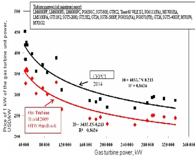
Figure 4: Price of gas turbines depending on power capacity
