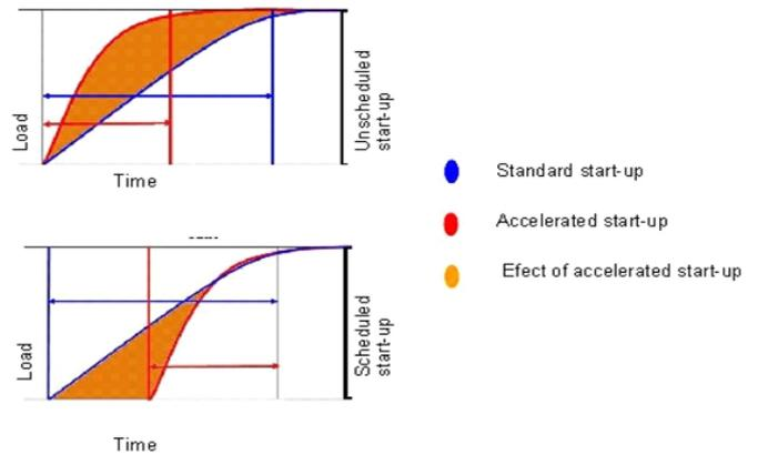
Figure 5: Accelerated start-up vs. standard start-up in the range of load and electricity generation
