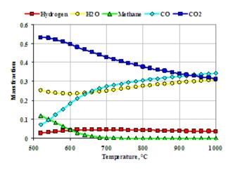
Figure 3: Wood Syngas composition as a function of temperature
