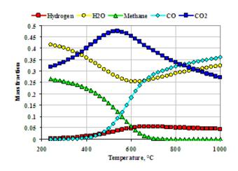
Figure 2: Canola Oil Syngas composition as a function of temperature
