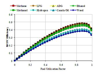
Figure 6: MCFC efficiency vs. fuel utilization factor for various biofuels
