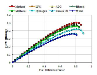
Figure 4: SOFC efficiency vs. fuel utilization factor for various biofuels
