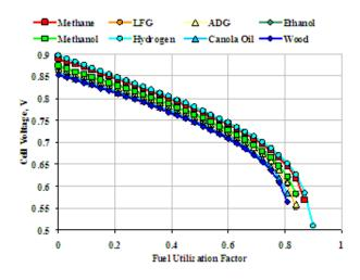
Figure 5: SOFC cell voltage vs. fuel utilization factor for various biofuels
