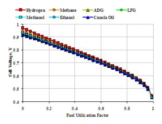
Figure 7: MCFC cell voltage vs. fuel utilization factor for various biofuels
