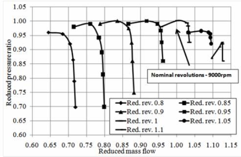
Figure 6: Example characteristic of reduced pressure ratio depending on reduced mass flow
