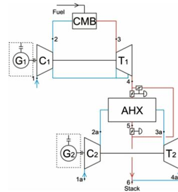
Figure 1: Reference gas turbine air bottoming cycle
