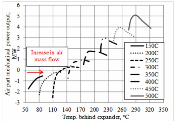
Figure 11: Power obtained by the air part for certain values of temperature after the air part expander
