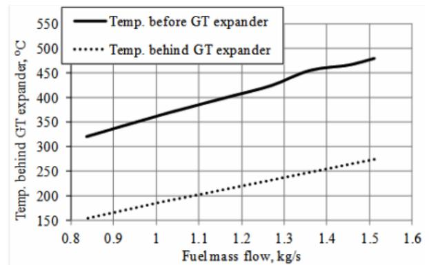
Figure 15: Temperature values before and after the air part expander for various values of fuel mass flow
