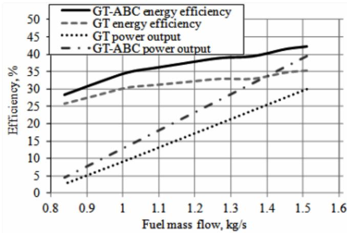
Figure 13: Increment in the gas-air system efficiency and mechanical power output
