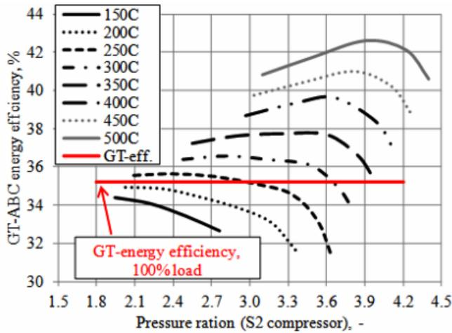
Figure 9: Gas-air system efficiency for different values of the pressure ratio of the air part compressor
