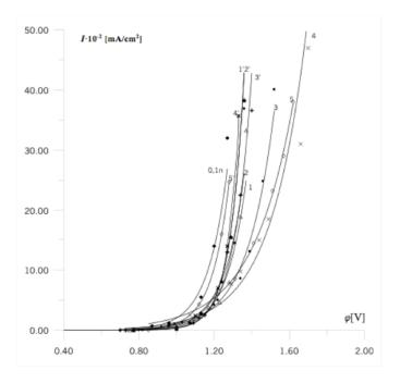
Figure 2: Polarization curves of electrooxidation of detergent SYNTANOL DS-10 (1'-5') and an emulsion of crude oil (1-5) in 0.1n concentration of electrolyte  $H_2SO_4$  (at 65°C): 1.1'-0.0025%; 2.2'-0.005%; 3.3'-0.010%; 4.4'-0.025%; 5.5'-0.050%
