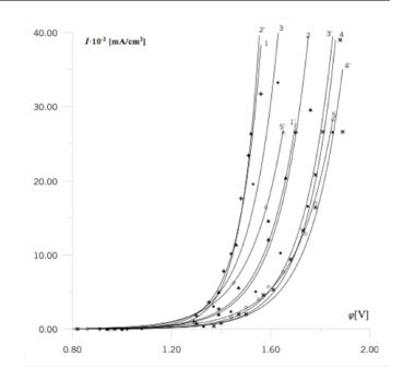
Figure 1: Polarization curves of electrooxidation of detergent SYNTANOL DS-10 (1'-5') and 0.01% emulsion of crude oil (1-5) in various concentration of electrolyte ( $H_2SO_4$ ): 1,1'-0.01N; 2.2'-0.05N; 3.3'-0.1N; 4.4'-1.0N; 5.5'-5.0N
