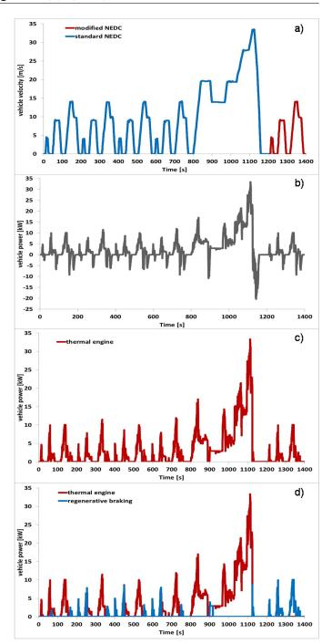
Figure 3: – a) standard and modified NEDC velocity schedules; b) resulting propulsive and braking powers; c) thermal engine power supply without KERS; d) thermal engine and KERS power supplies
