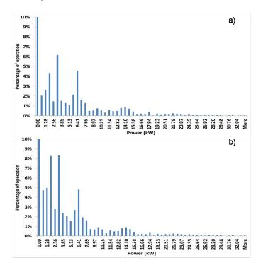
Figure 4: Percentage of the cycle the THERMAL ENGINE spends at a certain power without KERS (a) and with KERS (b)
