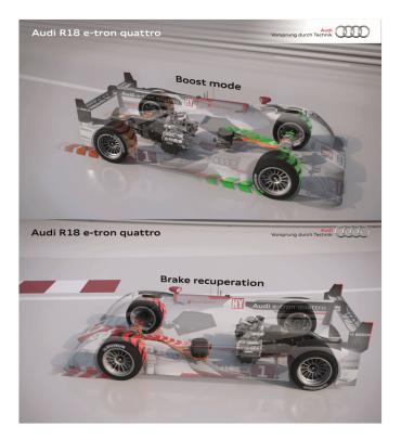
Figure 1: Audi R18 e-tron Quattro KERS (from [7]). Recuperation and boost mode of operation
