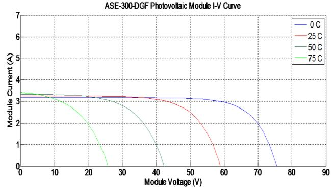
Figure 7: I-V curves (0.50 kW/m<sup>2</sup>; 0, 25, 50, 75°C)
