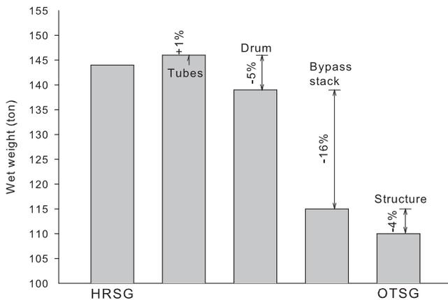
Figure 3: Breakdown of wet weight difference between a drum-type and a once-through HRSG for offshore applications
