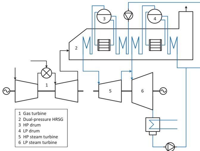
Figure 2: Simplified layout of onshore combined cycle with dual-pressure drum-type HRSG
