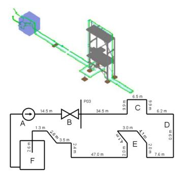
Figure 33: The experimental set-up of the PPP test ring [8]: A: Pump; B: Fast closing valve; C: Vertical bridge; D: Turning point; E: Vertical and horizontal bridge; F: Pressure tank B2
