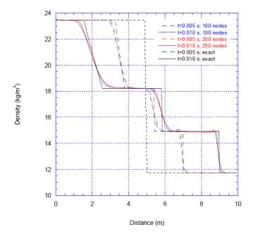
Figure 3: Air shock-tube—Riemann problem. Density profile, comparison of RELAP5 with exact solution
