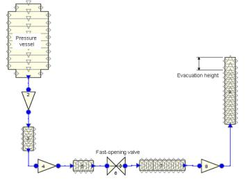
Figure 28: Nodalization of the CWHTF experimental facility
