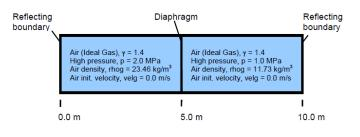
Figure 1: Schematic of air shock tube
