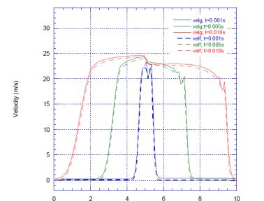
Figure 19: Two-phase shock tube. RELAP5 calculated profiles of phasic velocities at different times
