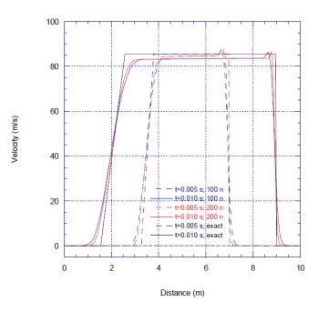
Figure 4: Air shock-tube—Riemann problem. Velocity profile, comparison of RELAP5 with exact solution
