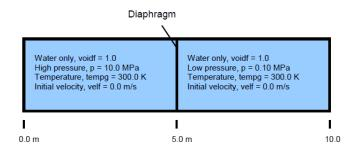
Figure 9: Schematic of single-phase liquid shock tube
