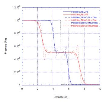
Figure 10: Liquid shock tube. Pressure profiles at different times, comparison of RELAP5 with DRAKO
