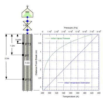
Figure 23: Pressurized pipe nodalization scheme with temperature and vapor pressure initial distributions
