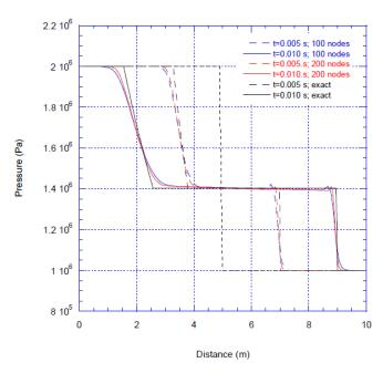
Figure 2: Air shock-tube—Riemann problem. Pressure profile, comparison of RELAP5 with exact solution
