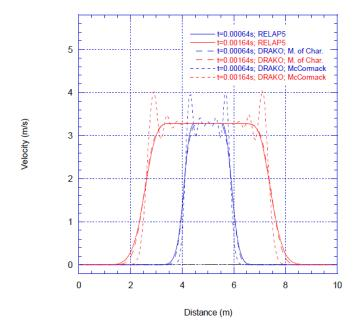
Figure 11: Liquid shock tube. Velocity profiles at different times, comparison of RELAP5 with DRAKO
