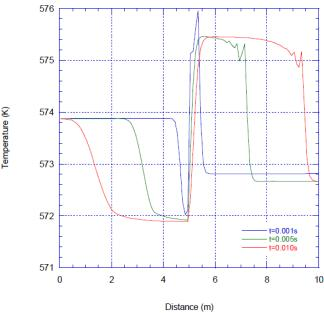
Figure 20: Two-phase shock tube. RELAP5 calculated liquid phase temperature profiles at different times
