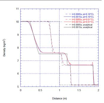
Figure 6: Water vapor shock tube. Pressure profile, comparison of RELAP5 with analytical solution
