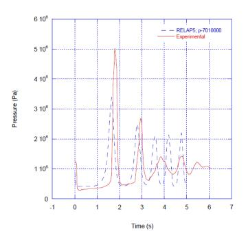
Figure 34: The UMSICHT test facility: pressure at P03
