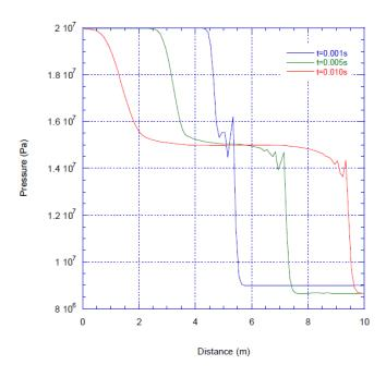
Figure 18: Two-phase shock tube. RELAP5 calculated pressure profiles at different times
