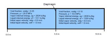
Figure 17: Two-phase shock tube problem initial conditions [13]
