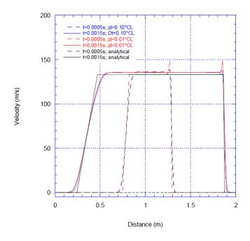
Figure 8: Water vapor shock tube. Vapor velocity profiles, comparison of RELAP5 with analytical solution
