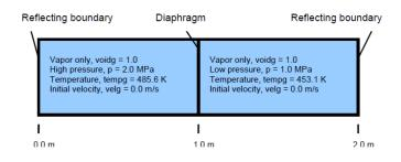
Figure 5: Schematic of single-phase vapor shock tube
