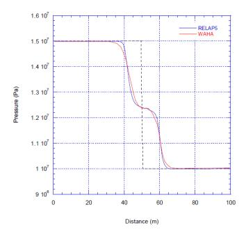
Figure 13: Two-phase shock tube. Pressure profile at time 0.0081 s, comparison of RELAP5 with WAHA
