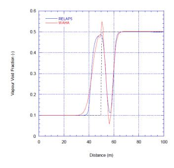
Figure 16: Two-phase shock tube. Vapor fraction profile at time 0.0081 s, comparison of RELAP5 with WAHA
