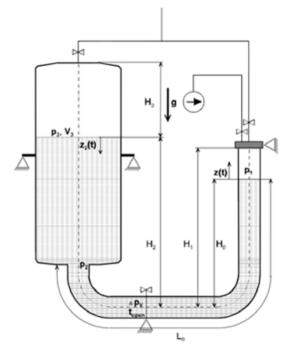
Figure 27: Schematic diagram of the CWHTF experimental facility
