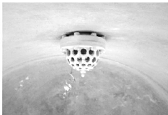
Figure 5: View of dispersing head mounted inside the test chamber
