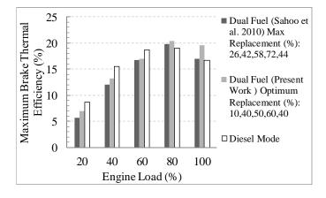
Figure 8: Comparison of maximum brake thermal efficiency between diesel and dual fuel modes
