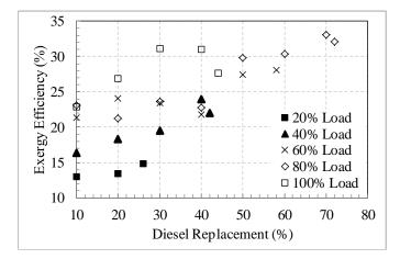
Figure 11: Variation of exergy efficiency with diesel replacement
