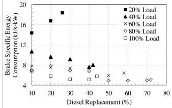
Figure 6: Variation of brake specific energy consumption with diesel replacement
