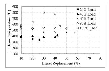
Figure 7: Variation of exhaust temperature with diesel replacement
