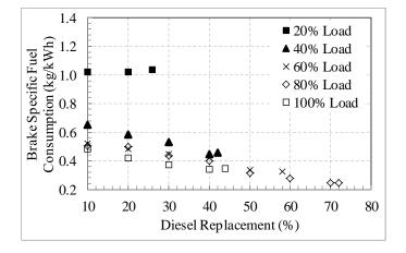
Figure 4: Variation of brake specific fuel consumption with diesel replacement
