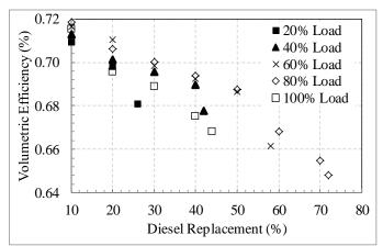
Figure 5: Variation of volumetric efficiency with diesel replacement
