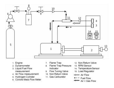
Figure 1: Schematic diagram of the setup
