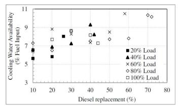
Figure 12: Variation of cooling water availability with diesel replacement
