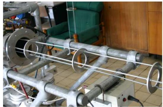
Figure 3: Schematic location of obstacles along the tube and the view of obstacles in the front of experimental tube
