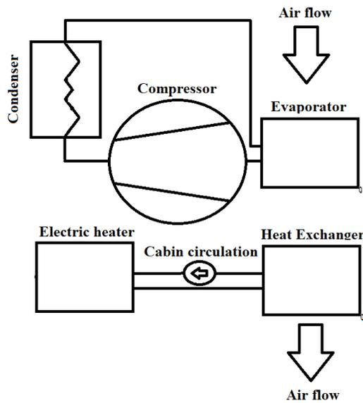
Figure 2: Tesla Model S heating-cooling system diagram (I II three-way valve)
