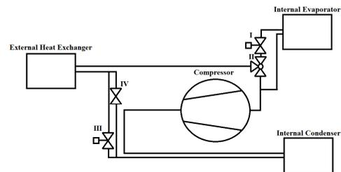
Figure 1: Nissan Leaf heating-cooling system diagram ( I III expansion valve, II three-way valve , IV bypass )
