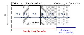
Figure 2: Thermal resistance model
