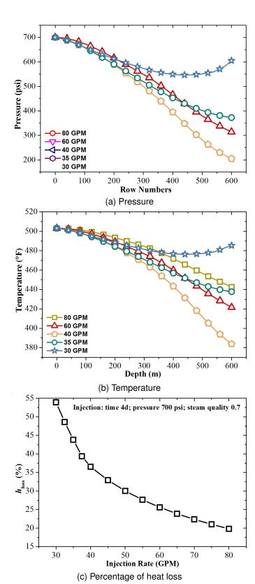
Figure 3: Effect of injection rate on wellbore thermal performance
