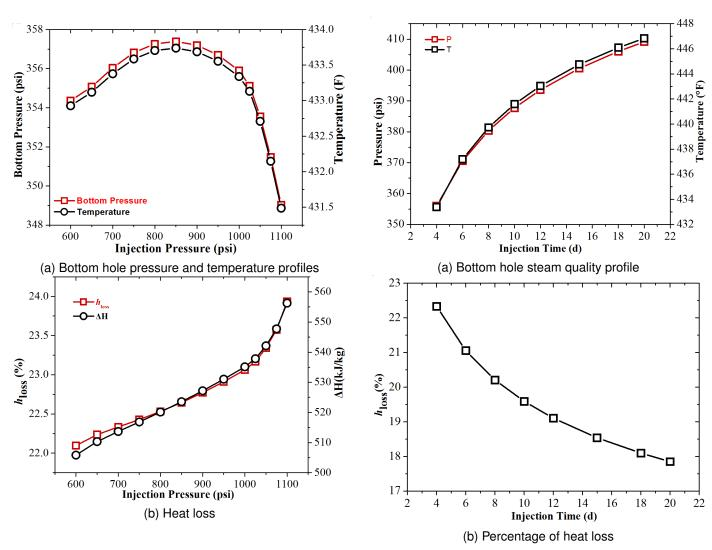
Figure 4: Effect of injection pressure on wellbore thermal performance
