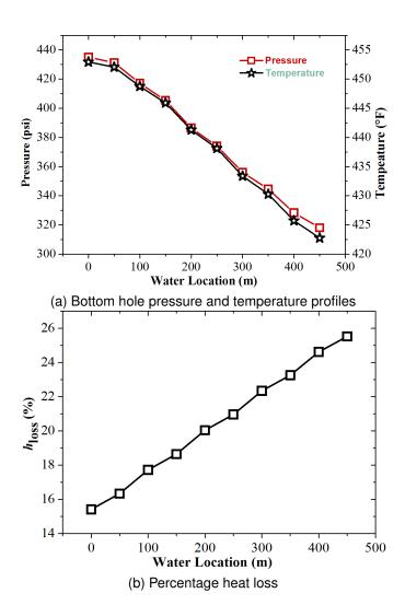
Figure 6: Effect of water in the annulus on wellbore thermal performance
