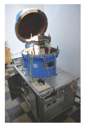
Figure 11: Stand for testing high-temperature fuel cells at Warsaw University of Technology
