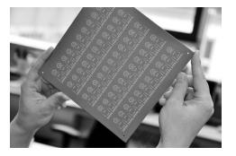
Figure 1: Large size  $(200 \times 200 \text{ mm})$ , low-temperature co-fired ceramic substrate with mass produced, highly repetitive, ceramic multilayer substrate size is the industry standard
