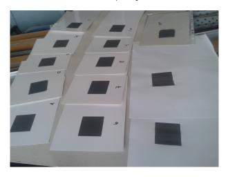
Figure 9: Molten Carbonate Fuel Cell cathode layers screen-printed on various substrates
