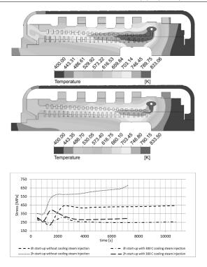
Figure 6: H-M-H stress course during turbine start-up
