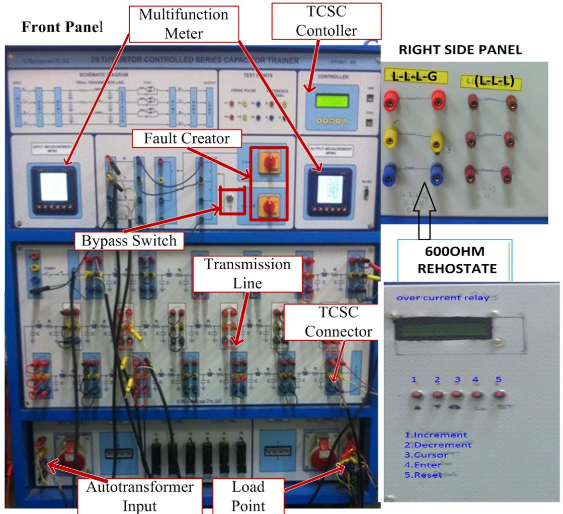
Figure 1: Prototype Model of TCSC Connected 180km long Transmission Line
