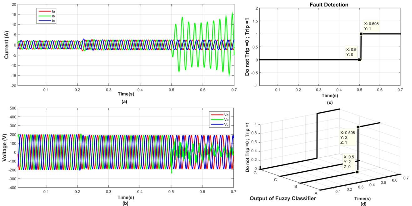
Figure 5: Performance during BG internal fault at near end (a) Current Signals (b) Voltage Signals (c) Fault detection (d) Fault classification
