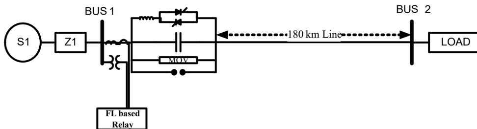
Figure 2: Single line diagram of TCSC compensated transmission network
