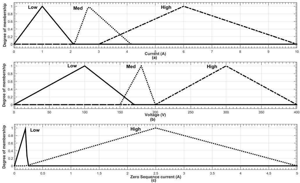
Figure 4: Degree of fuzzy membership function for input variable (a) current for phase fault detection (b) voltage for phase fault detection (c) zero sequence current for ground fault detection
