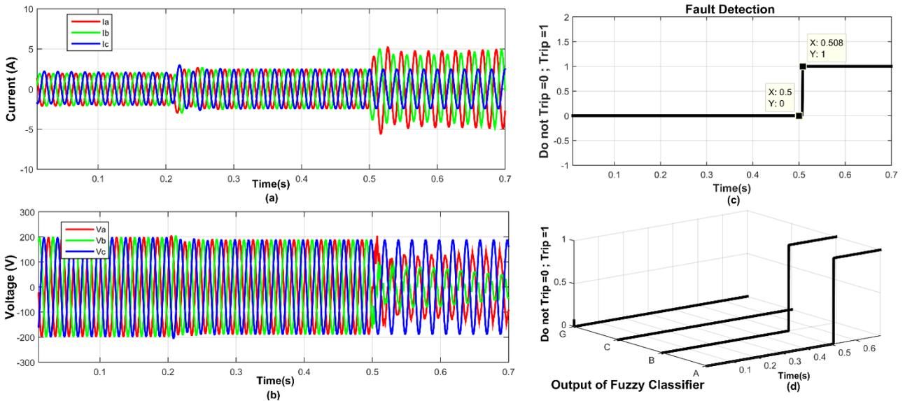
Figure 7: Performance during LL fault (a) Current (b) Voltage (c) Fault detection (d) Fault classification
