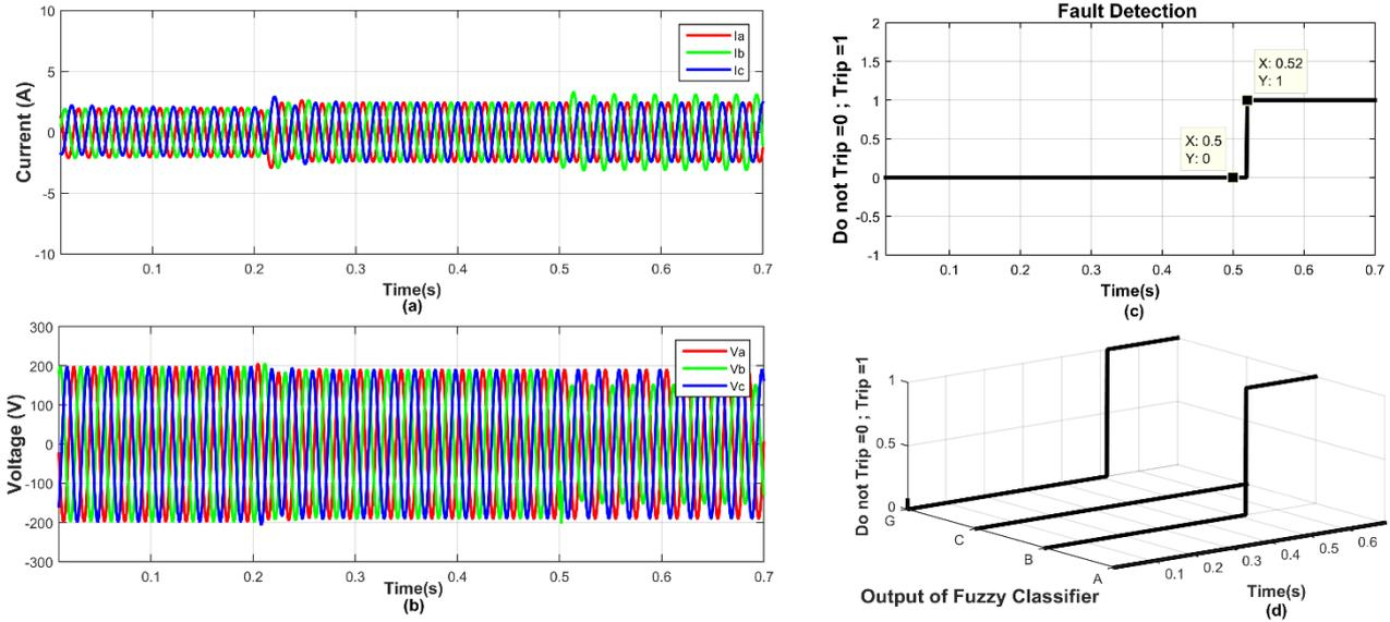
Figure 6: Performance during BG internal fault at remote end (a) Current Signals (b) Voltage Signals (c) Fault detection (d) Fault classification
