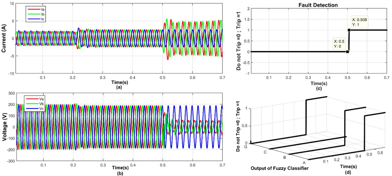
Figure 8: Performance during LLG fault (a) Current (b) Voltage (c) Fault detection (d) Fault classification
