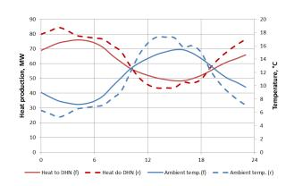
Figure 10: Comparison of forecast (f) and real (r) ambient temperature and heat demand for the analyzed day of CHP operation
