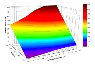
Figure 5: Net power output  $(N_{elGT})$  as a function of the gas turbine load  $(Q_{GT})$  and air inlet temperature  $(t_{am})$
