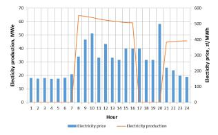
Figure 9: Results of hourly electricity production in CHP plant and electricity price changing during one day [13]
