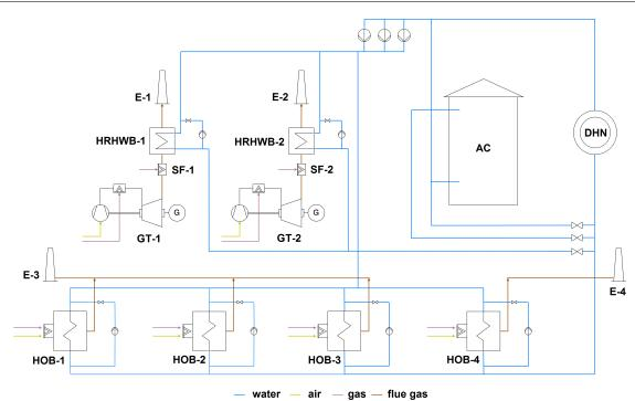
Figure 1: Schematic diagram of the gas fired cogeneration plant
