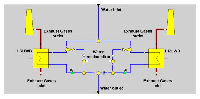
Figure 6: Part of the model with Heat Recovery Hot Water Boilers (HRHWB) system
