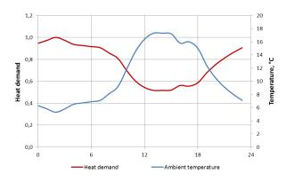
Figure 2: Graph showing an example of changing heat demand and ambient temperature during the day
