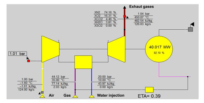
Figure 4: Gas turbine model using the characteristics utilizing vendor information in the form of correction curves
