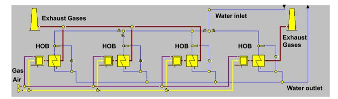
Figure 7: Part of the model presenting four Heat Only Boilers system (HOB)
