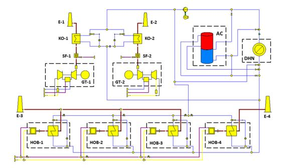
Figure 3: Schematic diagram of the mathematical model of gas fired plant: AC—Hot Water Accumulator, E—Emitter, GT—Gas Turbine, HOB—Heat Only Boiler, HRHWB—Heat Recovery Hot Water Boiler, DHN—District Heating Network, SF—Supplementary Firing System
