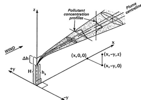
Figure 1: Gaussian plume from the elevated point source [2]
