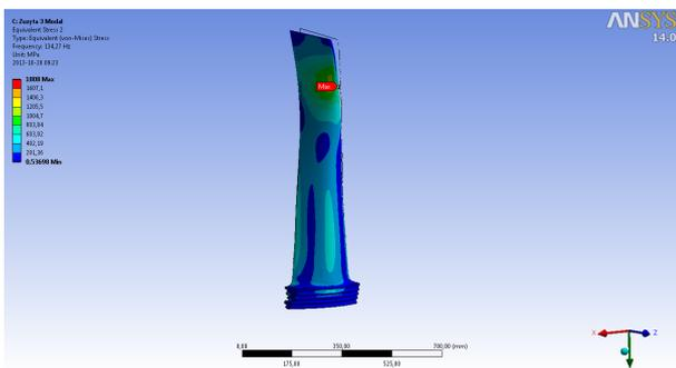
Figure 15: Stresses for the second form of own vibrations of the “moderately worn” blade
