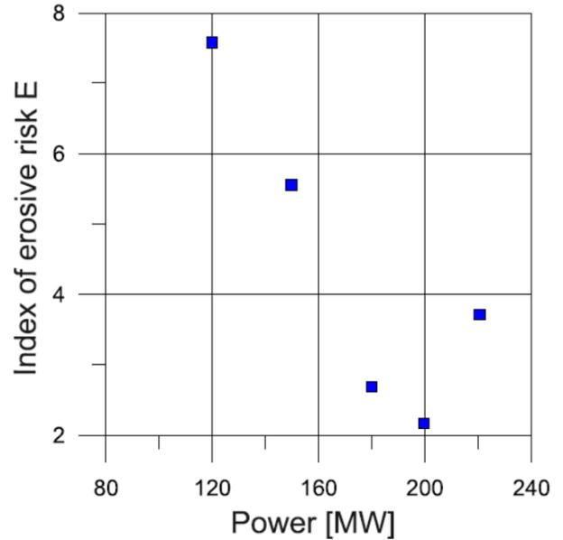
Figure 8: Erosion index for different load values turbine B
