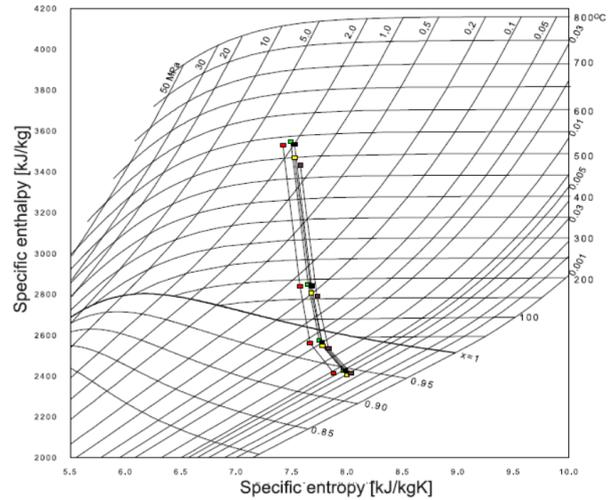
Figure 6: Expansion line in the IP and LP parts of the turbine B—red for the load of 220.56 MW, green for the load of 199.56 MW, black for the load of 179.87 MW, yellow for the load of 149.7 MW and brown for the load of 119.9 MW
