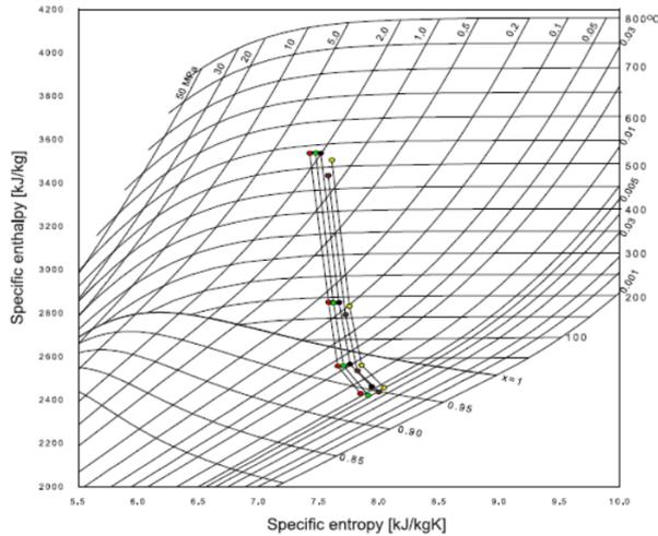
Figure 3: Expansion line in the IP and LP parts of turbine A—red for the load of 218.82 MW, green for the load of 199.92 MW, black for the load of 178.98 MW, yellow for the load of 139.12 MW and brown for the load of 119.42 MW
