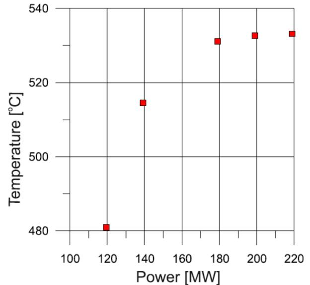
Figure 4: Temperature of re-superheated steam for different load values, turbine A
