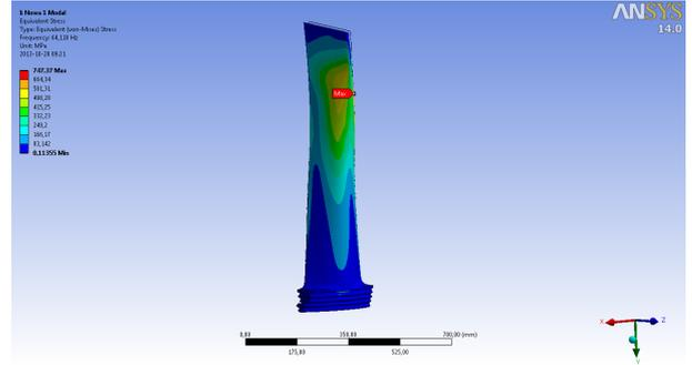
Figure 11: Stress for the first form of own vibrations of the “new” blade
