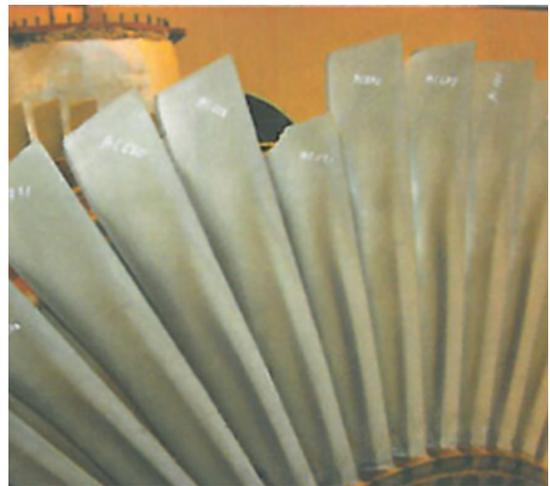
Figure 16: Rotor with a damaged blade
