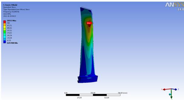
Figure 14: Stresses for the first form of own vibrations of the “moderately worn” blade
