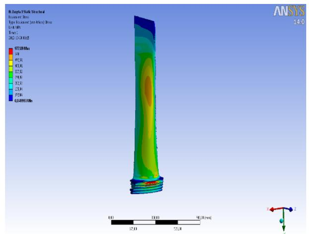
Figure 13: Stress in the “moderately worn” blade induced by rotation
