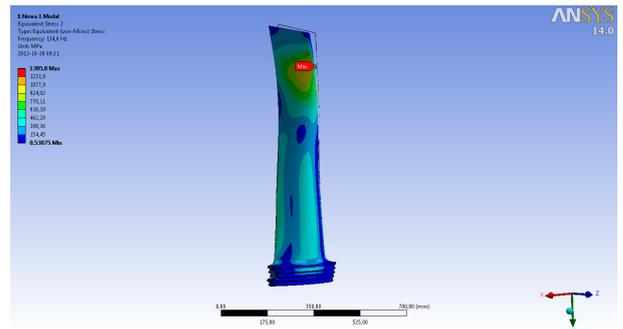
Figure 12: Stress for the second form of own vibrations of the “new” blade
