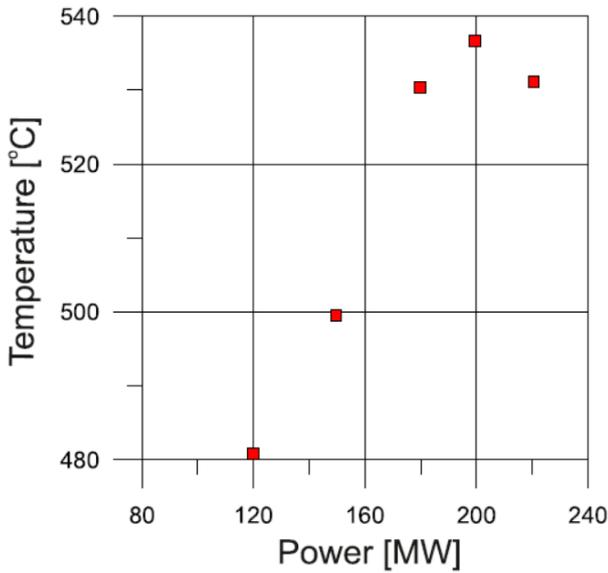
Figure 7: Temperature of re-superheated steam for different load values turbine B
