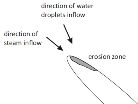
Figure 2: Direction of steam and water droplets inflow on the leading edge of the rotor blade
