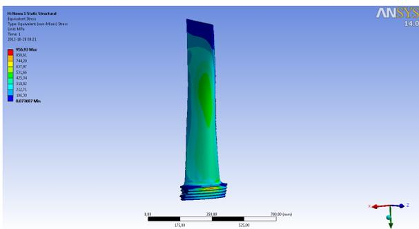
Figure 10: Stress on the “new” blade induced by rotation
