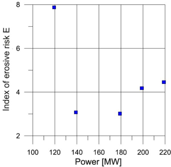
Figure 5: Erosion index for different load values turbine A
