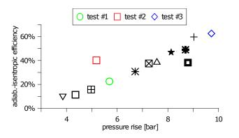
Figure 6: Adiabatic efficiency of the expander [8]
