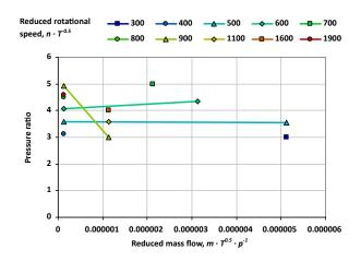
Figure 14: The expander operated on carbon dioxide pressure ratio as a function of reduced mass flow,  $\frac{\dot{m} \cdot \sqrt{T}}{p}$  for various reduced rotational speeds,  $\frac{n}{\sqrt{T}}$
