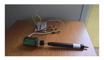
Figure 11: The expander-generator set used for the experiments
