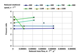
Figure 13: The expander operated on air pressure ratio as a function of reduced mass flow,  $\frac{m}{\sqrt{T}}$  for various reduced rotational speeds,  $\frac{n}{\sqrt{T}}$
