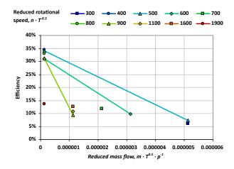
Figure 16: Efficiency curves for expander operated on carbon dioxide as functions of reduced mass flow,  $\frac{m}{\sqrt{T}}$  for various reduced rotational speeds,  $\frac{n}{\sqrt{T}}$
