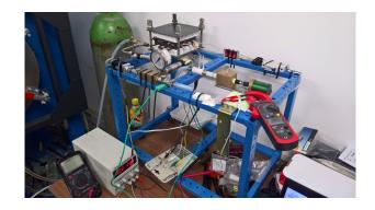
Figure 12: The test stand for characterization of micro rotary sliding vane expander opaerated on  $\mbox{CO}_2$
