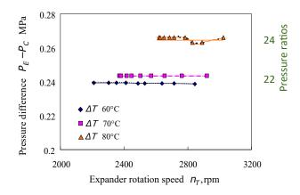
Figure 1: The influence of temperature difference on pressure difference as a function of expander rotational speed [4]
