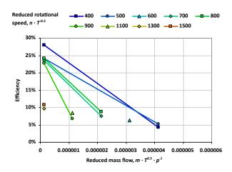
Figure 15: Efficiency curves for expander operated on air as functions of reduced mass flow,  $\frac{m}{\sqrt{T}}$  for various reduced rotational speeds,  $\frac{n}{\sqrt{T}}$
