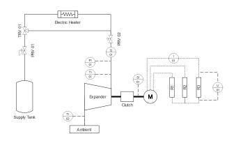
Figure 9: Simplified schematic of the laboratory stand for characterization of rotary sliding vane expander
