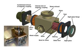
Figure 4: Design of the vane expander [7]
