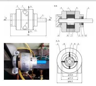
Figure 7: A general view and simplified construction scheme of the expander [9]
