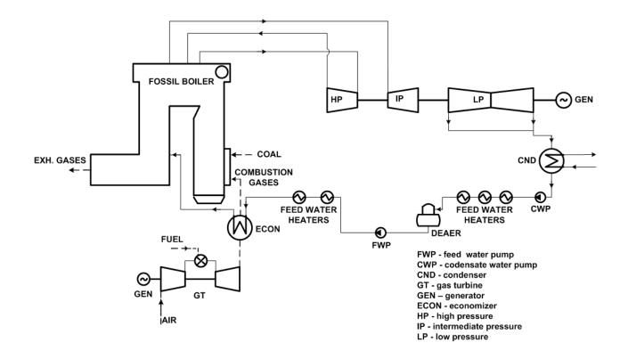
Figure 3: Pre-cooling hot windbox application
