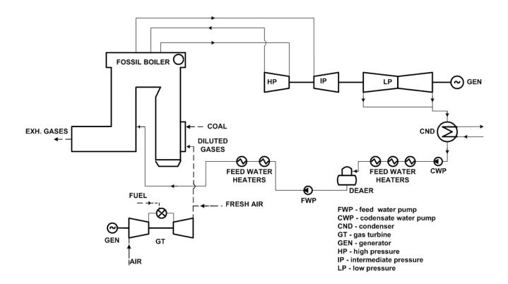
Figure 2: Fresh air dilution hot windbox repowering
