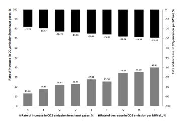
Figure 10: Rate of increase in CO2 emission in exhaust gases and decrease in CO2 emission per MW electrical power
