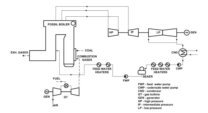
Figure 1: Direct hot windbox repowering
