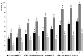
Figure 6: Variation of GT power ratio, rate of increase ST and CCPP power after repowering
