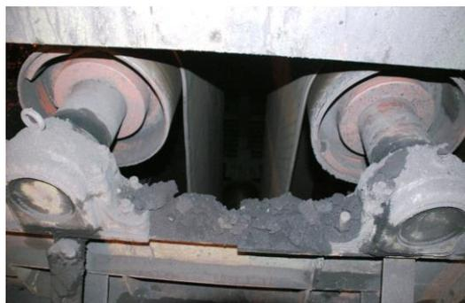
Figure 9. Bend pulleys
