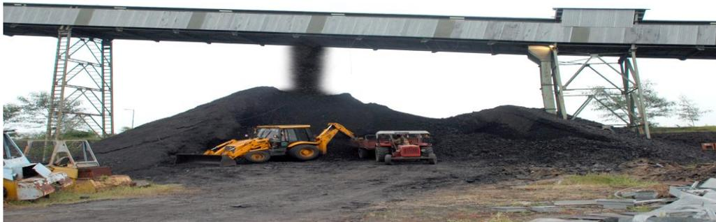
Figure 6: Free fall of coal on ground after installation of wiper
